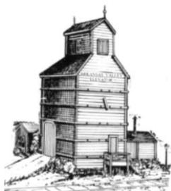
The elevator was a place where the farmer stored his grain after it was harvested. After the grain was dumped into the floor grate, the cups (in the window) carried it to the storage bins overhead. The farmer could either sell the grain right after harvesting, or he could store it at a later time, hoping that he could sell it for a higher price at a later time.
